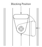
Once stop is set into position opposite side to glass insertion point, the other side is then rotated to the stop position.
