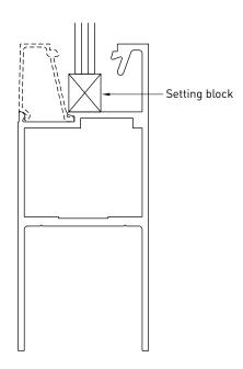
One setting block is placed under glass. The glass adjusting screw, right, is then wound down to come in contact with the top of the glass, keep winding until the stile rises up to the correct position.
