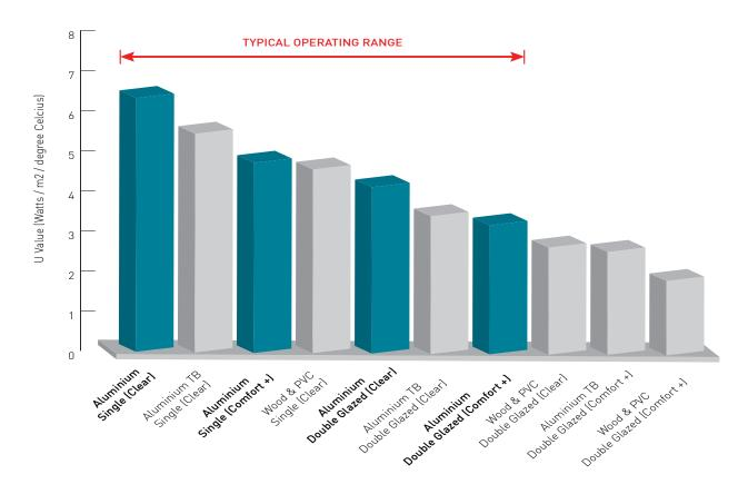
In addition to optimising the U value there are two other factors that will need consideration- the solar heat gain coefficient (SHGC) and visible transmission (VT). The ideal values will depend on whether the building is located in either hot or cold climates. In selecting glazing options there are a number of options that can be considered:
