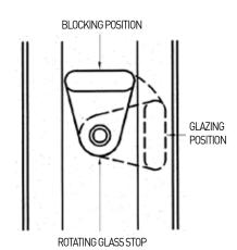
Once stop is set into position opposite side to glass insertion point, the other side is then rotated to the stop position.
