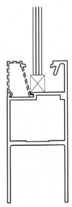
The glass adjusting screw, right, is then wound down to come in contact with the top of the glass, keep winding until the
